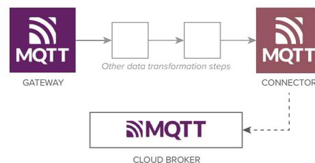
This approach permits a high volume request response pattern, but requires the use of two different MQTT endpoints. Very similar to Gateway to Channel approach, except facilitates high volume egress as well.
