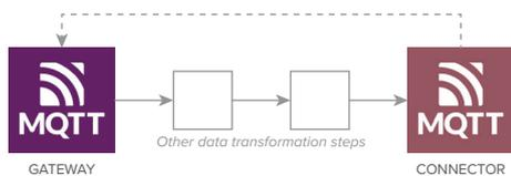
This is a naive implementation of a request response pattern over MQTT. Data is published to a Topic on the Gateway, and the Connector is publishing to other Topics on the Gateway, to which the consumer is subscribing. Auto-scaling on the MQTT Gateway can mean that some messages may be published on different replicas and therefore may not be able to be reliably subscribed to.
