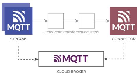
This approach permits a high volume request response pattern, but only if topic segregation is possible (for example with Sparkplug B). It permits the use of a single MQTT endpoint for both request and response.
